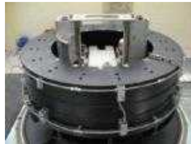
Drum Centrifuge, 1.2m (Dia.) (University of Western Australia, COFS)
