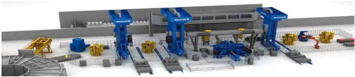
그림 176 Forging and rolling railway wheels in a complete system
