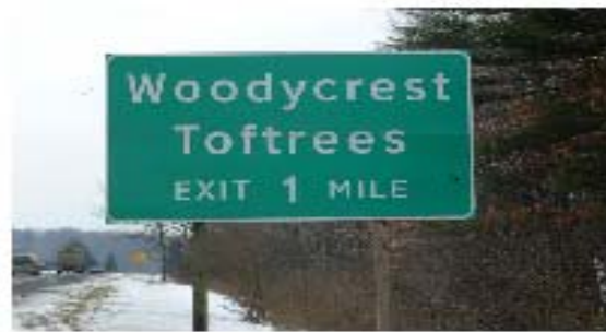
Example of a sign near Penn State that uses the new Clearview road sign typeface based on University research.
