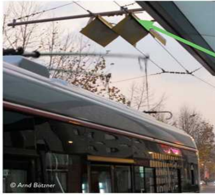
▶ Un-wiring and re-wiring with connection funnel on Shanghai's route 71 BRT, taking less than 5 seconds
