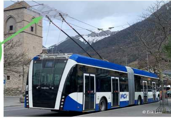
▶ Transparent funnels in Villeneuve, Switzerland, are less visually intrusive
