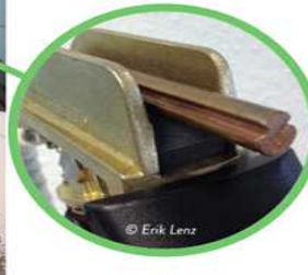
Vehicle current collector head with copper overhead wire.
