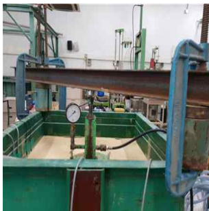
(e) Reaction beam installation
