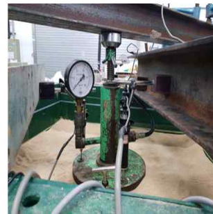
(f) LVDT installation
