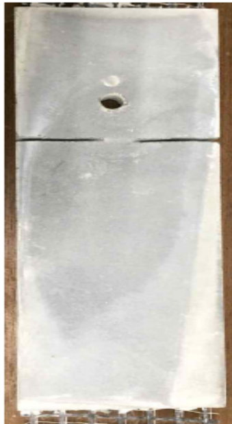
양생 후 saw cutting
