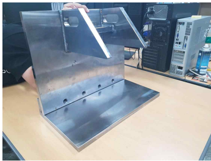
(a) Reaction Bridge (Jig)
