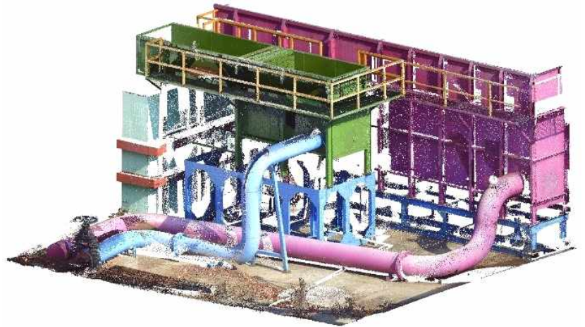
< KICT water treatment facility and its LiDAR scanned pre-processed point cloud data >
