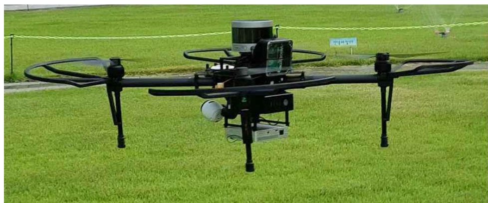
< Fully equipped Matrix 100 UAV with 1,079g payload >
