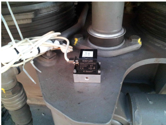
Fig. 2 Vibration Acceleration Sensor of Bogie
