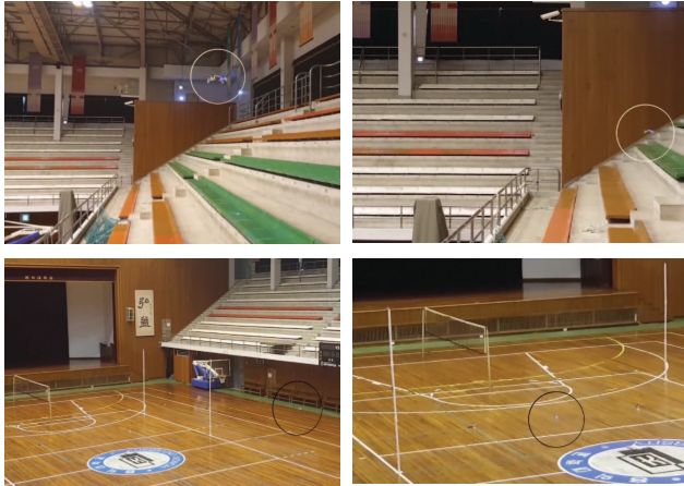
Figure 2. Experiment on a fixed-wing UAV landing route using a test bed for flight test. A Crazyfly (quadcopter) is located around the center of the circle.
