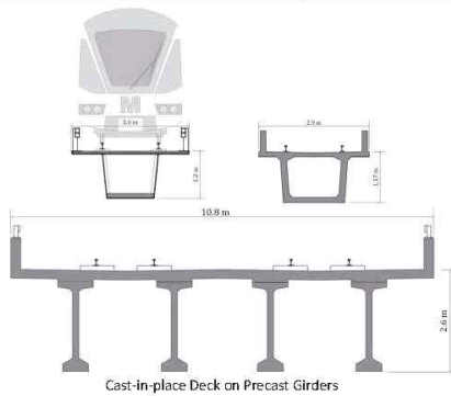
Cast-in-place Deck on Precast Girders
