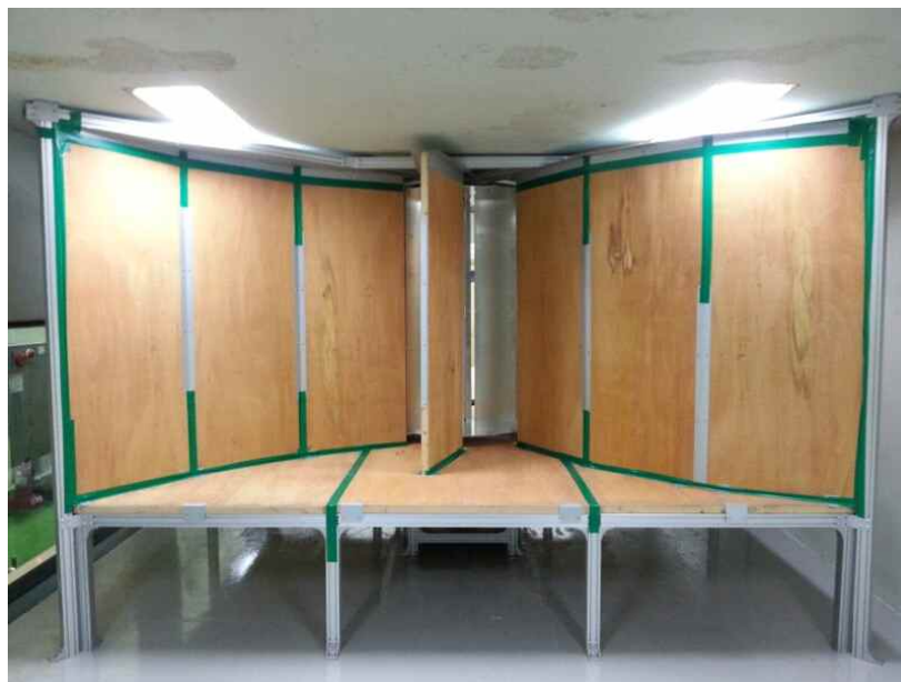
<그림 76> The model wind turbine system with the guide vanes and turbine impeller installed at the test section of the subsonic wind tunnel.
