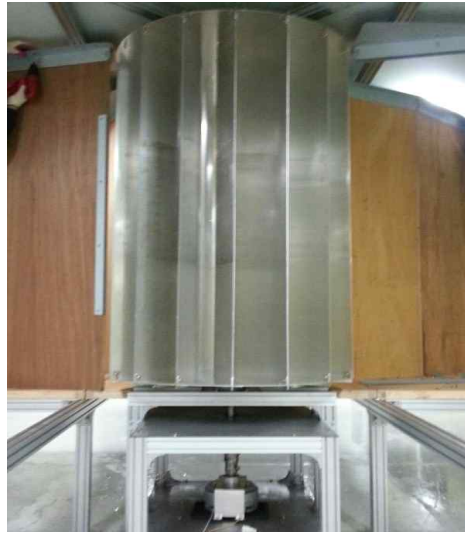
<그림 78> The model turbine impeller assembled with 16 blades and mounted on the test bed.
