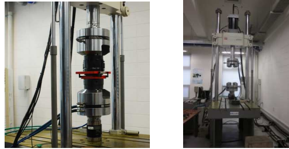
Fig. 3 Dynamic test of the bearing using a UTM
