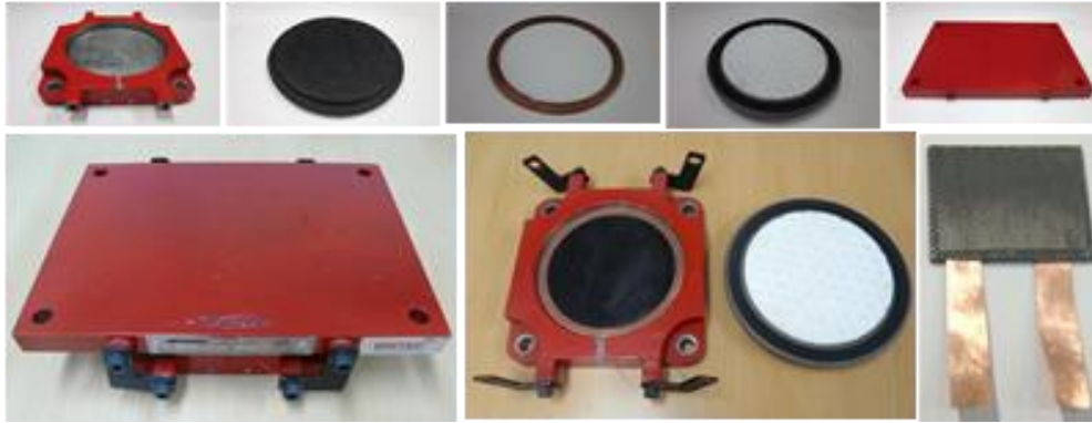
Fig. 1 Pot bearing and its components (pot plate, elastomeric disc, brass sealing ring, piston with PTFE, slide plate) and PCGE used in the tests
