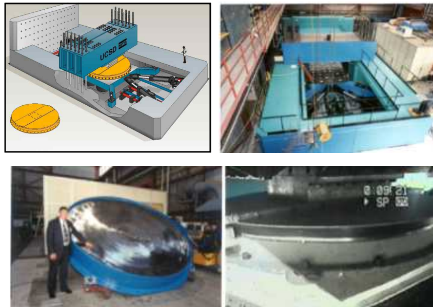
〈MAURER-SOEHLNE Friction Pendulum Sliding Bearing Test〉
