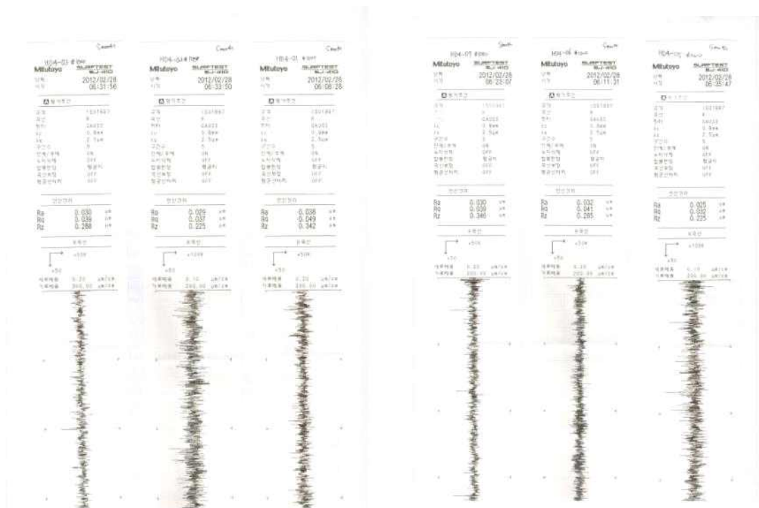
[Surface roughness test results of SSRT specimen]
