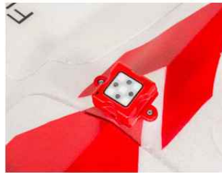
DLS(Downwelling Light Sensor)
