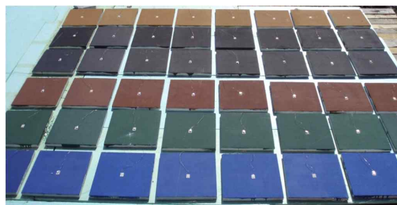
(그림 3.15) Tested tiles coated with common, cool and PCM coatings (Source: Karlessi, 2011)
