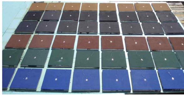
(그림 6.11) Tested tiles coated with common, cool and PCM coatings (Source: Karlessi, 2011)
