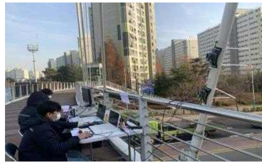
(a) A Bridge Cable Tension Measurement
