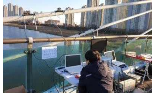
(b) B Bridge Cable Tension Measurement
