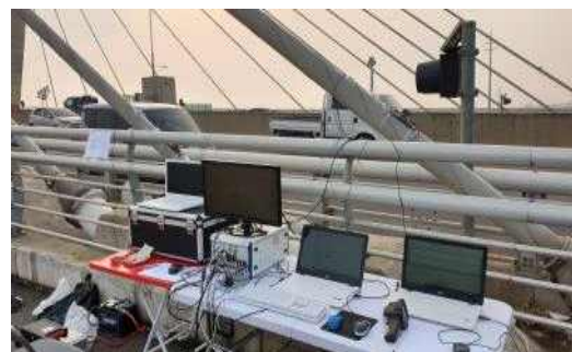
(e) E Bridge Cable Tension Measurement
