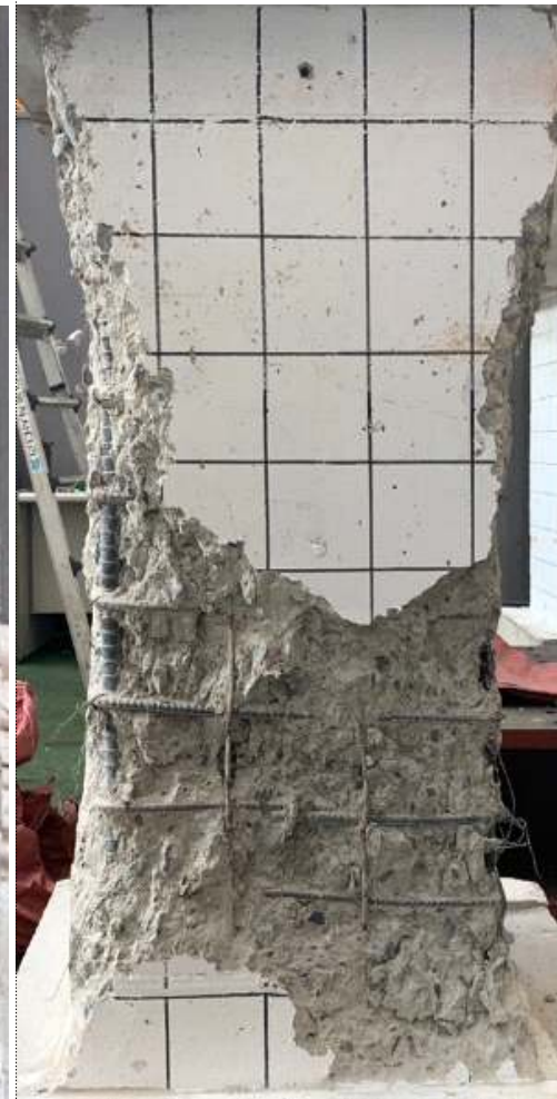
(c) Section maintain strengthening ( 1.0 A_{sh} )
