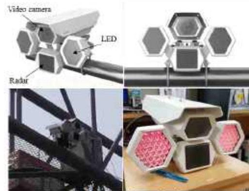
Fig. 4. Proposed system hardware
