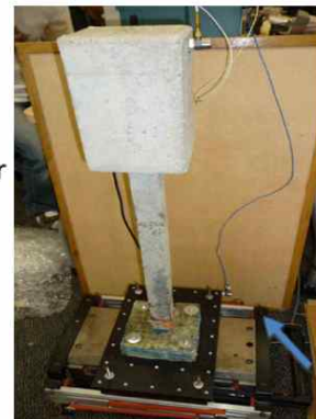
Fig. 10. Seismic shaking table test setup.
