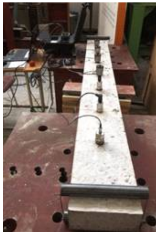
(b) Installation of sensor
