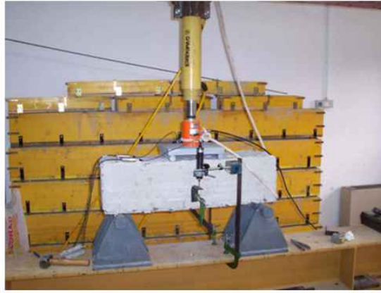
Fig. 6a. Set-up for flexural tests – coarse aggregates replaced by rubber particles.
