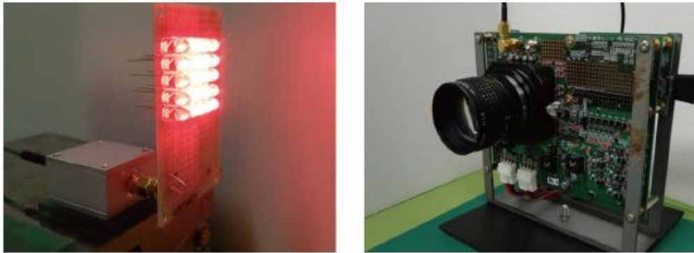
그림 5 OCI-based VLC system. (a) 4 \times 5 LED array transmitter. (b) Camera receiver.
