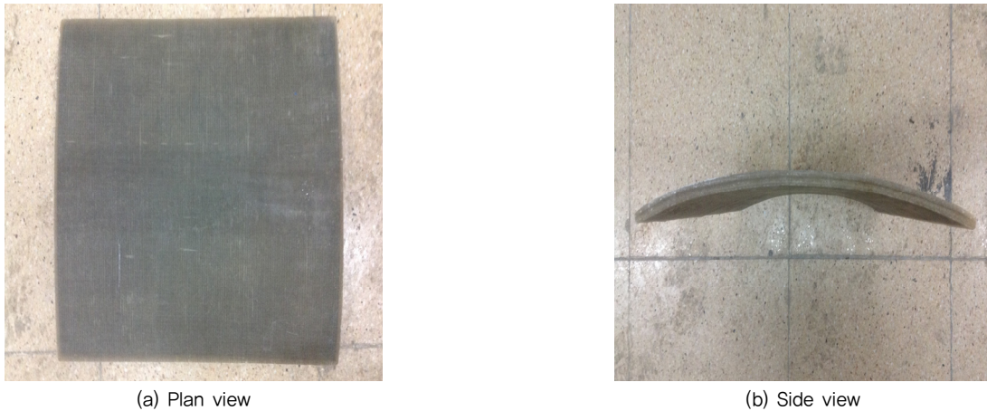
Fig. 4 Photo of hybrid steel/GFRP panel gate
