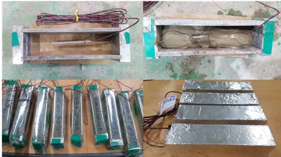
Fig. 8.2 shrinkage test set-up
