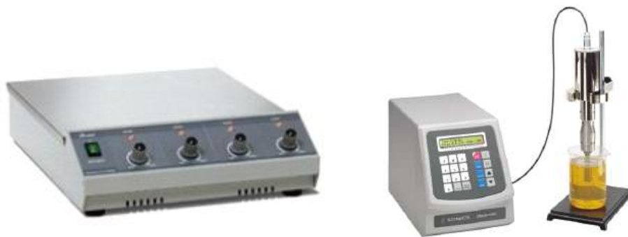
Fig. 2.2 Magnetic stirrer & Ultrasonic process
