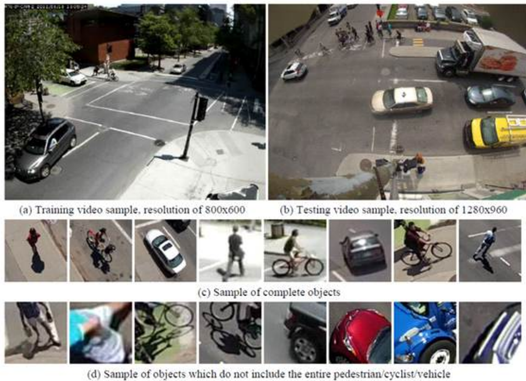
Figure 2. Sample of extracted road user images used for training and testing
