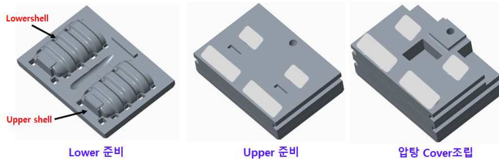
(a) Upper shell, Lower shell Mold size : 774x538x318(WxDxH)
