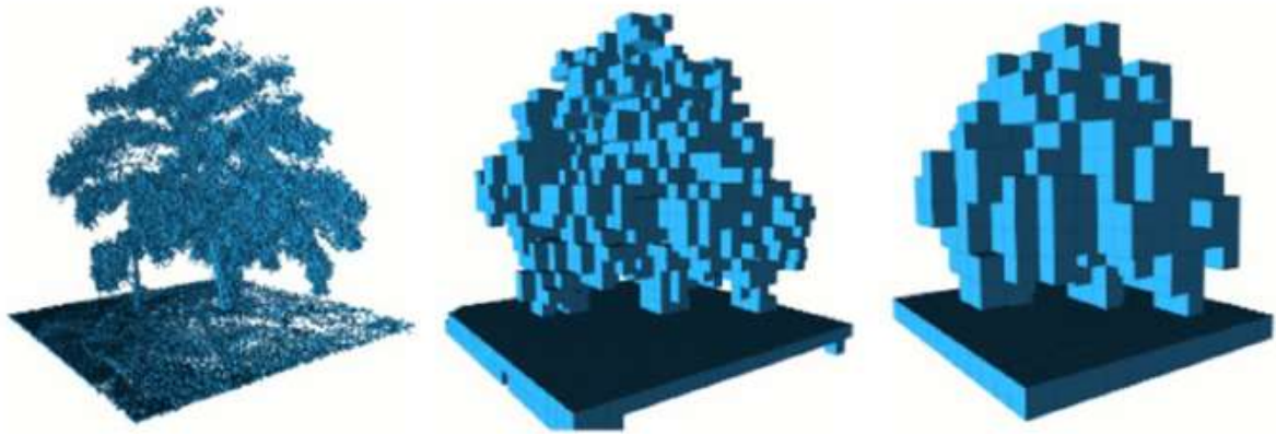
그림 86 Occupied voxels represented by different resolutions 0.08m, 0.64m, 1.28m respectively
