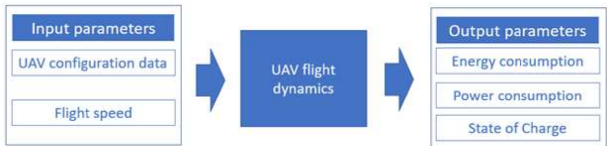
그림 70 Energy consumption, power consumption and state of charge estimation method
