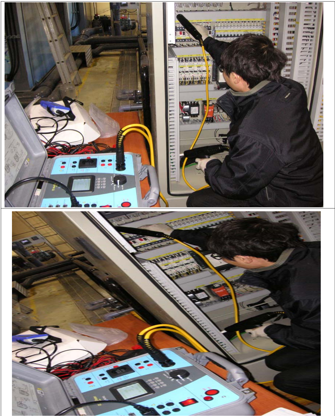
[그림 3.3.1] High Voltage Test(According to sub-clauses 19.4 of EN60204-1)
