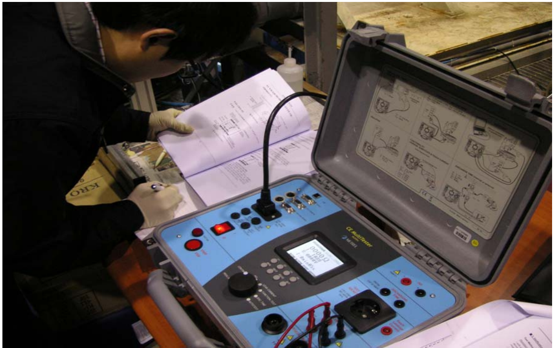
[그림 3.3.3] Insulation Test (According to sub-clauses 19.4 of EN60204-1)
