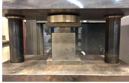
(b) Compression of specimen
