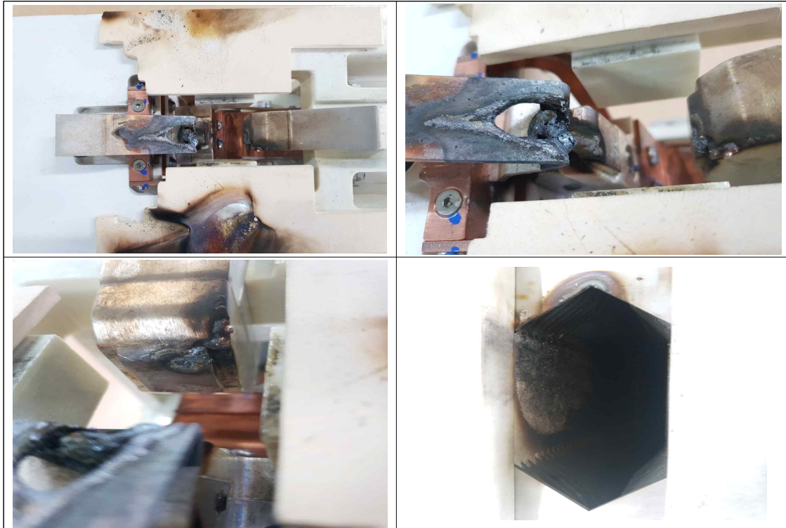
(2) Photo 2 : Test object after the breaking test of DC 1,800[V], 250[A] (Serial Number : 1VC1BL00032883)
