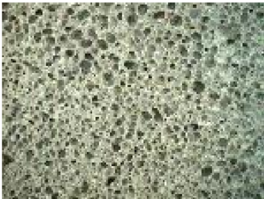
(e) Sodium silicate 40% + \text{CaCO}_3 1%
