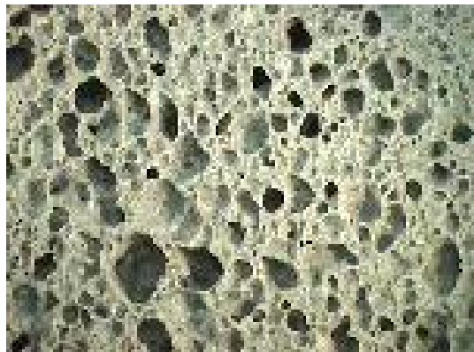
(f) Sodium silicate 40% + \text{CaCO}_3 2%
