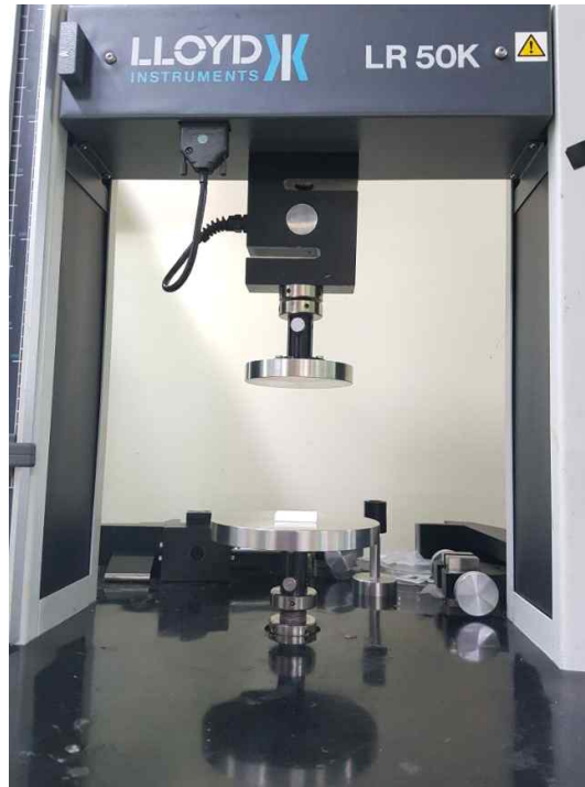
Fig. E16 UTM(universal test machine) used for mechanical strength measurement of PET-PEN copolymer.
