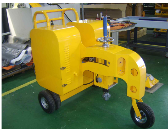
(a)Portable Impact Seismic Source 측면
