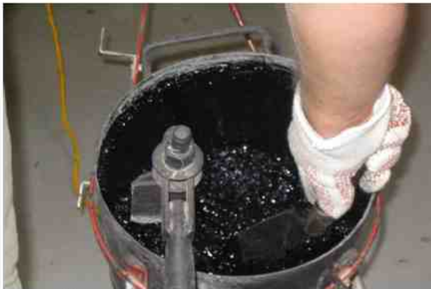
Figure 4. Warm Mix Asphalt in Bucket Mixer
