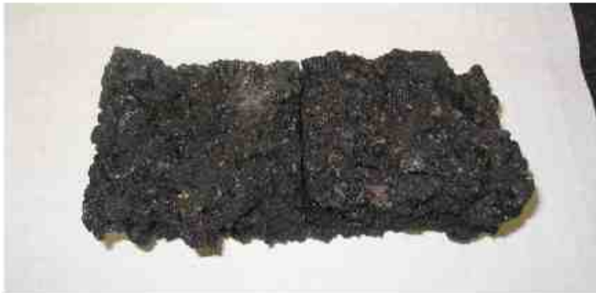
Figure 14. Example of Cohesive Stripping Failure – Granite
