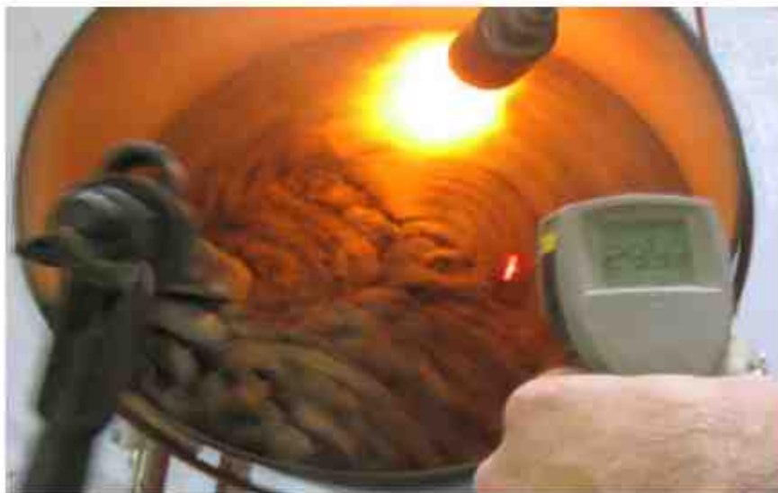
Figure 3. Heating of Wet Aggregate to Mixing Temperature
