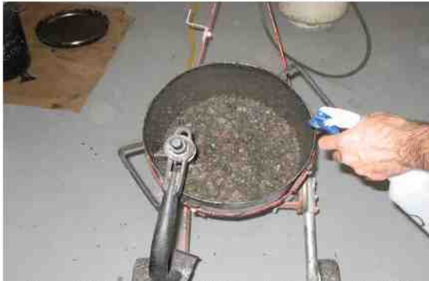
Figure 2. Introduction of Moisture to Aggregate for TSR Samples
