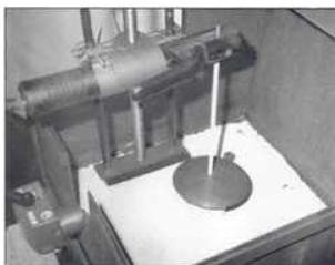
welding equipment setup showing the SMAW electrode and the rotating copper disk
