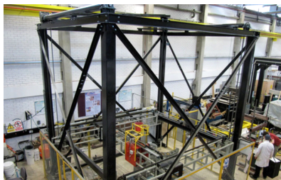
(a) Concrete Printing system
